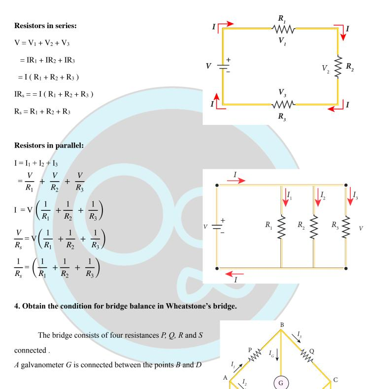
When the points *B* and *D* are at the same potential, the bridge is said to be balanced.
