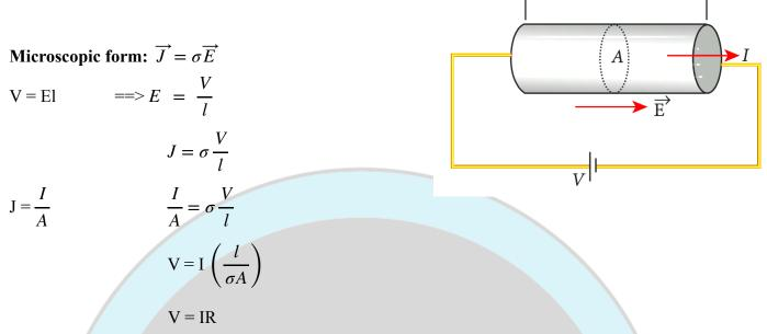
The resistance is the ratio of potential difference across the given conductor to the current passing through the conductor.
